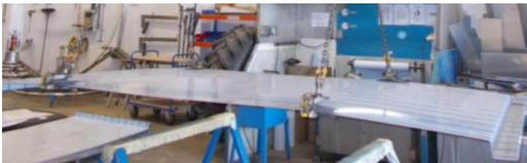
The formation of the gutter section of this thin sheet has increased the lateral stiffness but not the axial. The use of protective packing should not be used. The THS clamps were replaced by special non marring versions.
