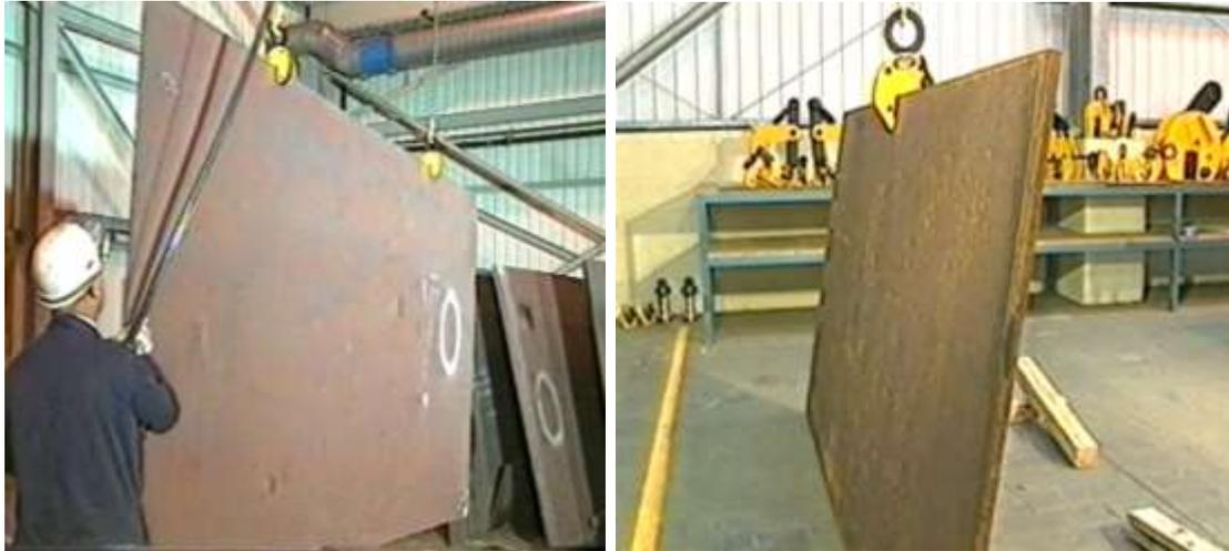
These two plates are the same length and width. The 30mm thick plate on the right can easily be handled by a single clamp. However to control the flexure of the 8mm plate on the left, 2 clamps have been used with a lifting beam.
